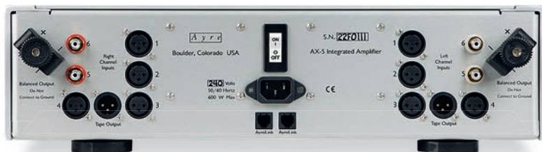
ABOVE: Cardas speaker terminals are joined by four balanced and two single-ended line inputs, plus tape out XLRs. The RJ-11 sockets provide 'AyreLink' system comms
